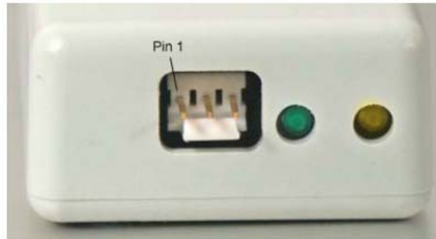
RS485 Connection View
