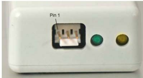
RS485 Connection View
