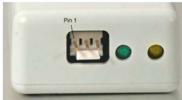
RS485 Connection View
